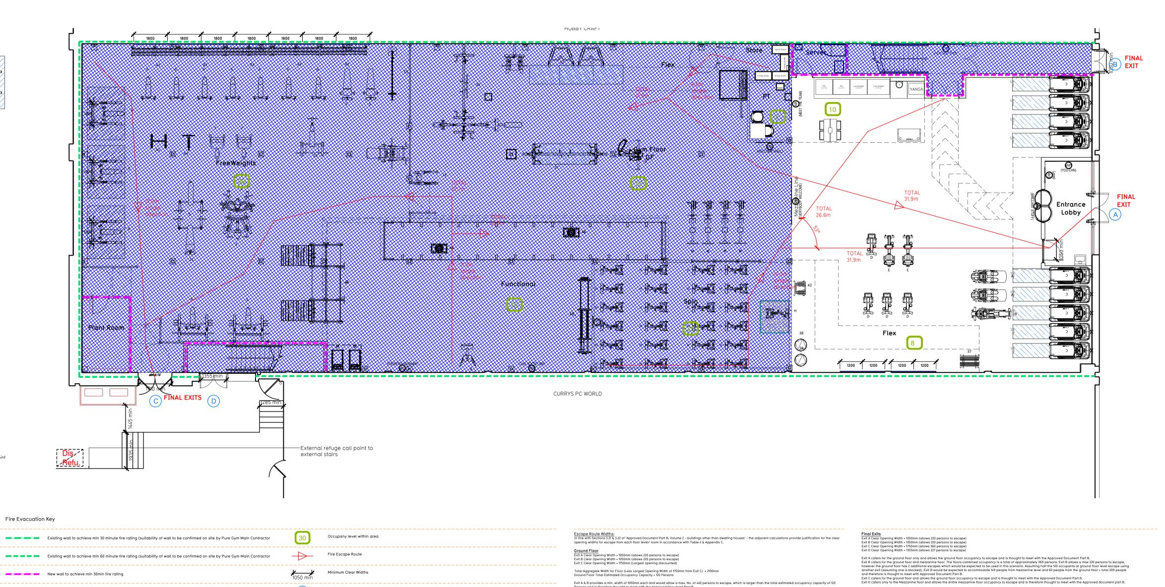
Exit A & B provides a min. width of 1050mm each and would allow a max. No. of 440 persons to escape, which is larger than the total estimated occupancy capacity of 120
